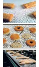
Rexnord® 505 MatTop® chain features a 0.5 in (12.7 mm) pitch and small 2 times width inside radius ideal for small packed food products. A 10% open area makes it also suitable for unpacked, fragile products needing careful handling on inline transfers. Rexnord<sup>®</sup> PosiTrack™ Tracking Guides offer stability and guidance. Rexnord® RBP and RB materials available.
